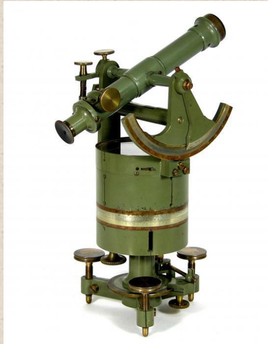
Pantômetro com bússola, parafusos calantes e luneta com círculo vertical (fonte: https://www.dehilster.info/pages/images/20th_c_pantometre_a_lunette_20170106095839b.jpg )
